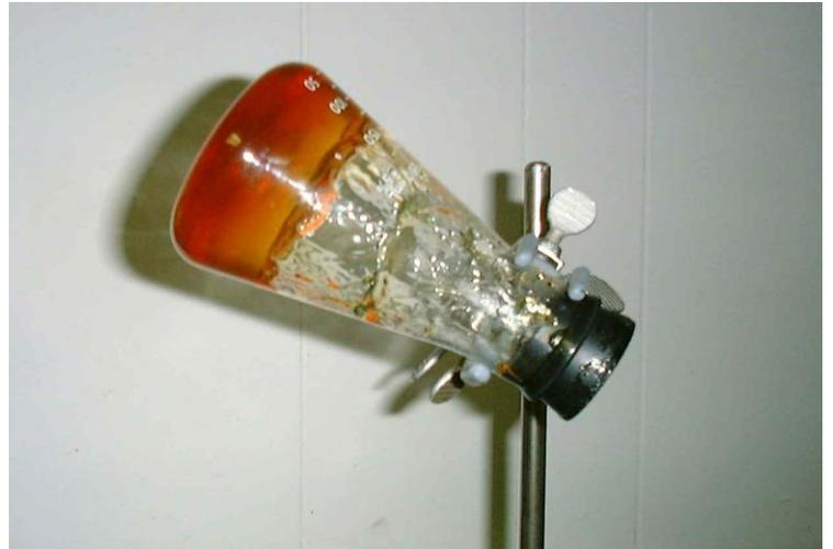
Isoparaffin oils generally have very good oxidation stability because of the characteristics of their synthetic base oil. Synthetic isoparaffins age more slowly than conventional petroleum based oil. This is partially due to the range of chemicals found in petroleum oil and the lack of impurities in synthetic base oils. Heat transfer fluids using isoparaffin oils contain added antioxidants to lengthen the service life of the product.
